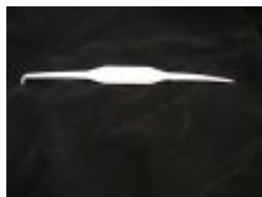
Trimming tool for casting & clay work similar to lacy with bent one edge
